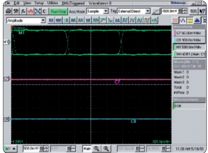
► Figure 3. 1.5 Gb/s signal with no probe loading.
